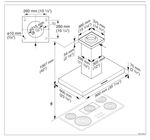
1) Opening for exhaust duct and power cord
